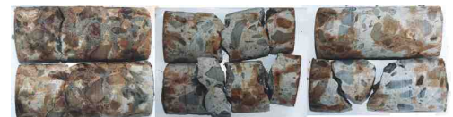
写真-2 浸透状況(呈色状);B2(注入圧力=0.5MPa)
